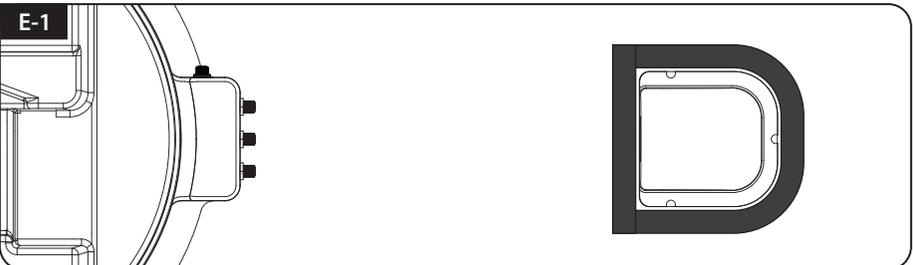
Place cable holder 30cm away from the rear centre of the antenna. Apply electrical tape 5mm from the outside of the holder
