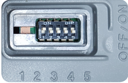
Dip switch image of the Multistacker. Set as dip switch 1 ON for NSW as an example.
