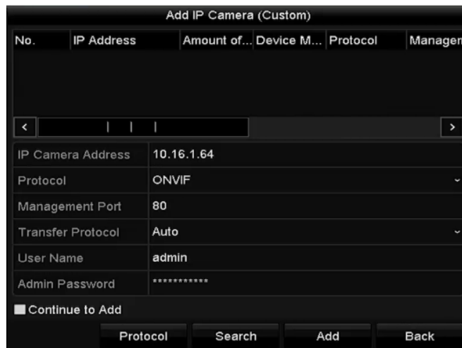
Figure 2. 31 Custom Adding IP Camera Interface
